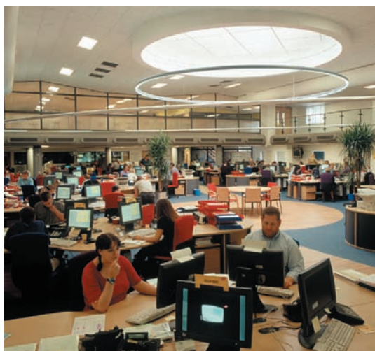
The illuminance levels vary between 300 and 1,300 lux throughout the day with the colour temperature varying between a warm 2,800K and a cool 5,300K.
